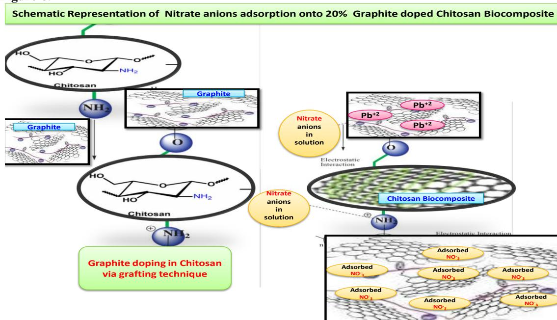
**Figure-8: Adsorption phenomenon of nitrate anions onto graphite doped chitosan**
