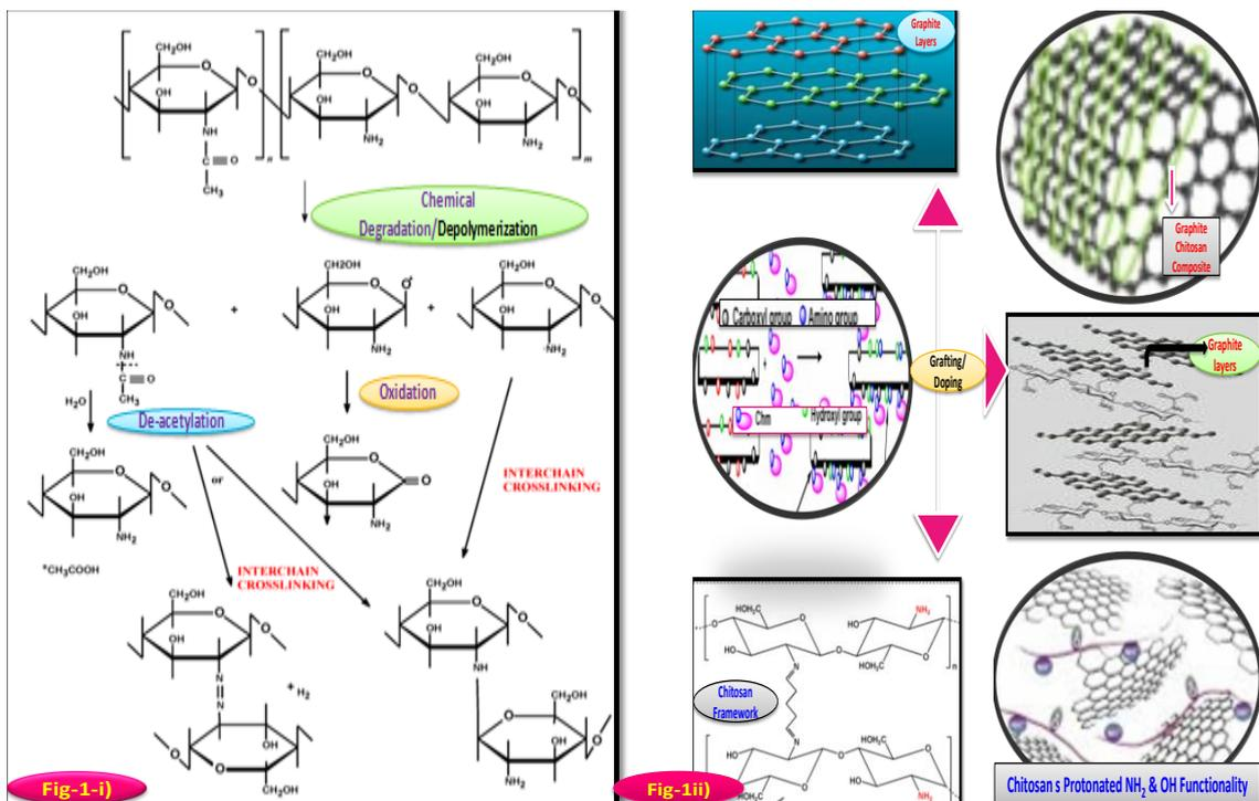
Fig-1: Preparation scheme i) chitosan treatment ii) 20% graphite doped chitosan bio-composite (5 mm).
