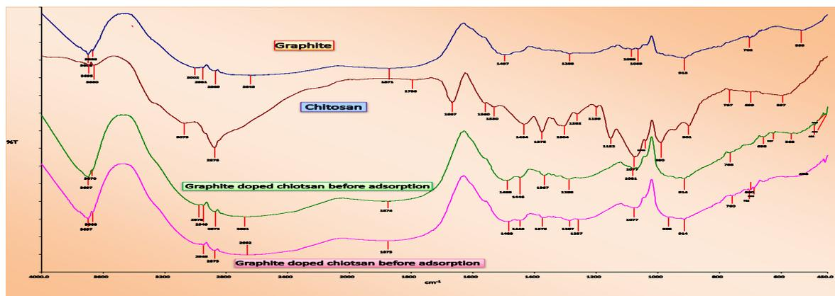
Figure-5: FTIR spectrum of (a) graphite, (b) chitosan, (c) Graphite doped chitosan composite before adsorption (d) Graphite doped chitosan after adsorption.
