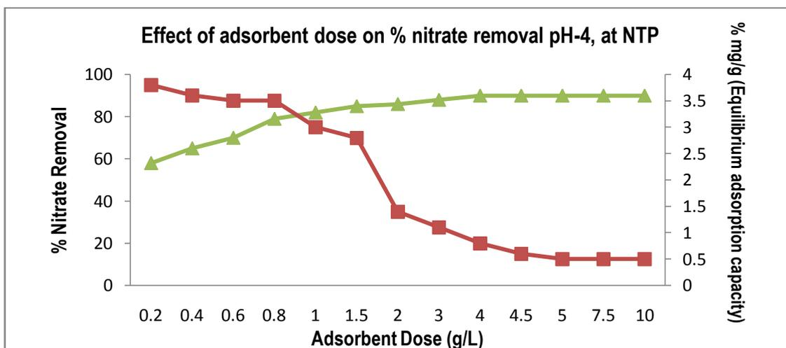
Figure-7: Effect of adsorbent dose on nitrate removal from water at NTP.
