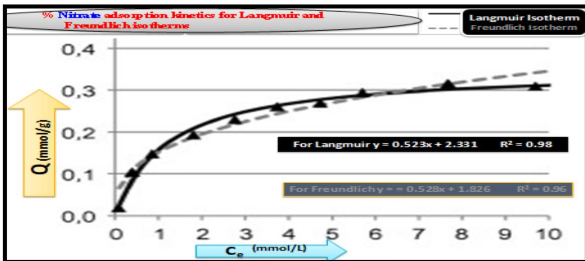
**Fig-2:** Langmuir and Freundlich adsorption isotherms plots for nitrate removal from water.
