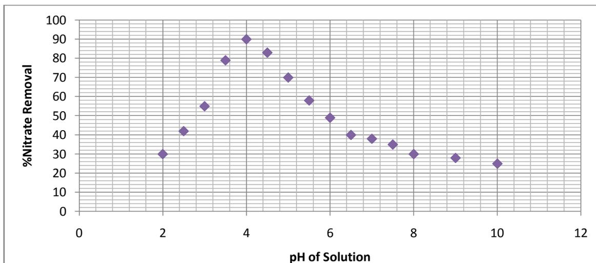
Fig-6: pH effect on effective nitrate sorption onto graphite doped chitosan biocomposite
